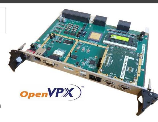
The board is provided together with an FMC mezzanine board (GR-VPX-SPW-MEZZ) which provides two SpaceWire interfaces on the front panel.
